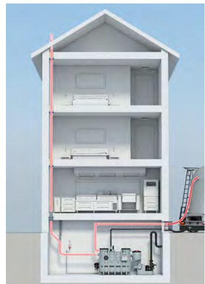
Pendulum gas line connected to grease separator
