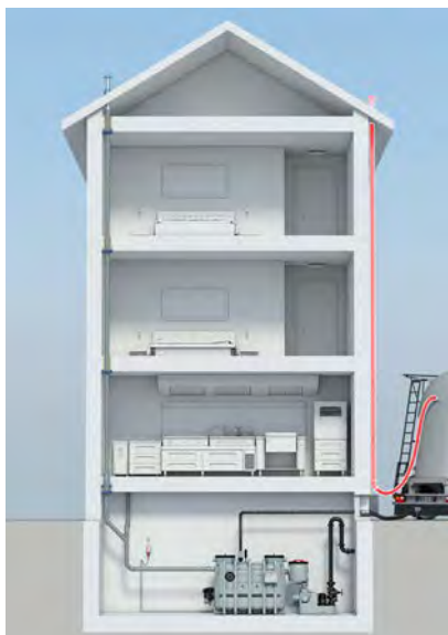
Separate pendulum gas pipe above the roof
