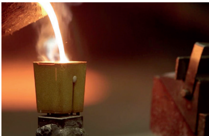
Sampling of cast iron for quality assurance
