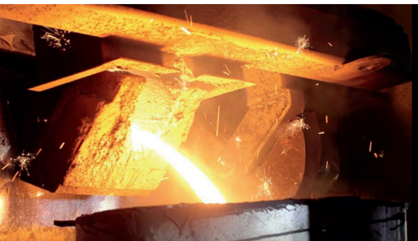
Molten cast iron in an electric furnace
