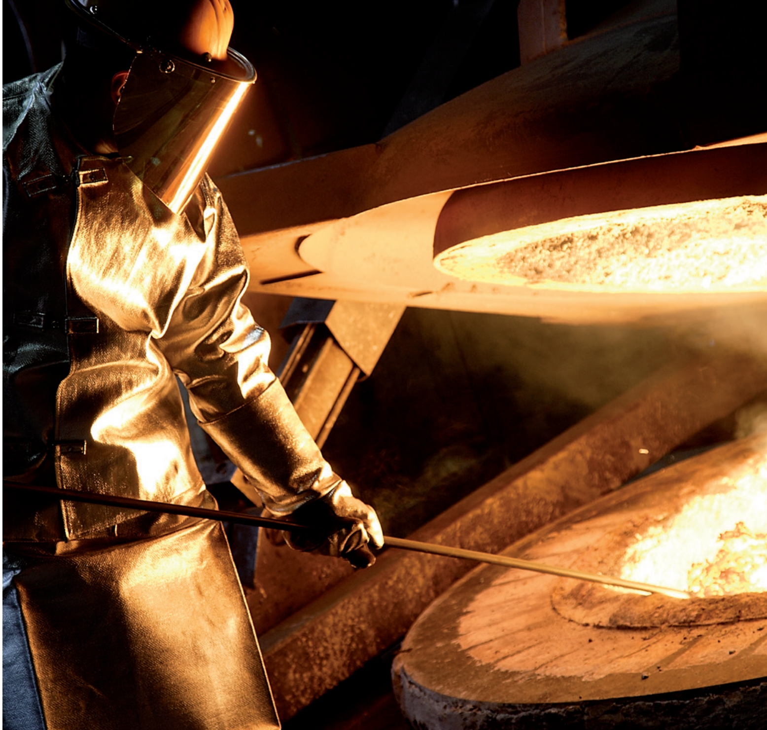
Sampling of the molten mass for spectral analysis
