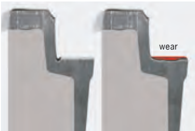
On the left, a section through a new frame On the right, a section through the identical type of frame after years in use
