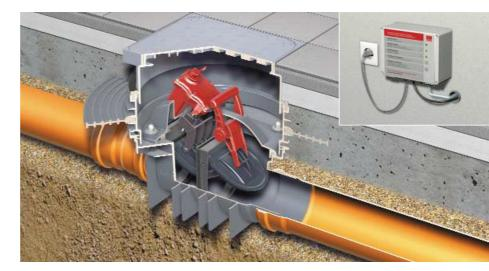
ACO QUATRIX®-K black water automatic backflow stop, DN 100 Type 3F pursuant to EN 13564 for installation in floor plates. Figure shows the ACO black water automatic backflow stop with the optional sealing flange to protect against pressurised water.
