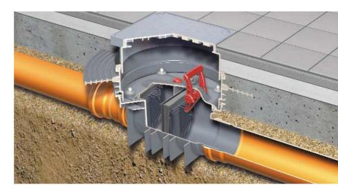
ACO TRIPLEX-K-2 double backflow stop, DN 100 Type 2 pursuant to EN 13564 for installation within floor plates. Figure shows TRIPLEX-K-2 with optional sealing flange to protect the device against pressurised water.
